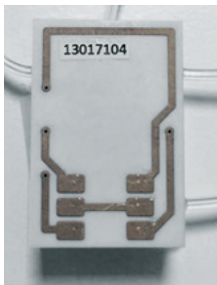
Figure 2: image of the back of the BioPAT Trace biosensor
